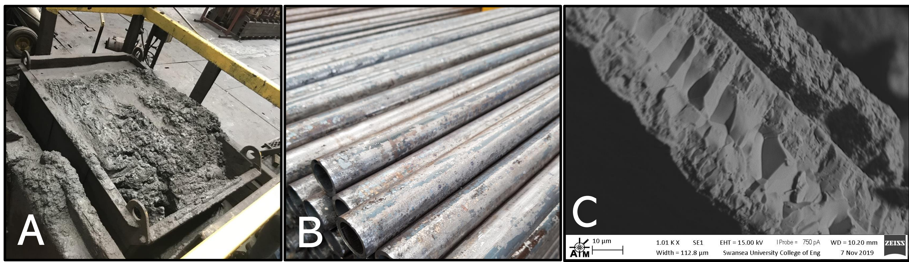
Figure 2a - Oxide waste containing quality grade steel (yield loss) Figure 2b - Surface cosmetic issues due to the normalisation scale Figure 2c - SEM Image cross sectional view of scale taken from process mill
